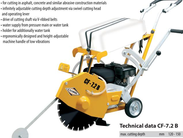
The new joint cutter CF-7.2 B achieves a good cutting performance in asphalt, concrete and in similar abrasive construction materials. It is especially appropriate for minor road repairing and for garden and landscaping. Easy handling and compact dimension make this machine ideal for rental business. Its compact construction ensures maximum flexibility during cutting and during transport, which makes the CF-7.2 B an ideal machine for repair jobs in areas narrow and of difficult access .
